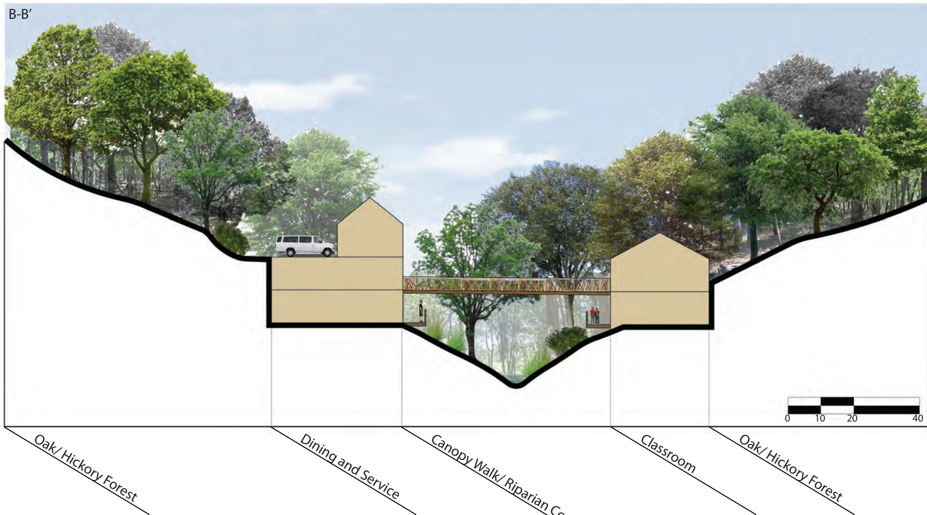
Section B-B' shows the canopy walk that connects the dining hall to the classroom building across the valley. Parking for service vehicles is located on the roof of the dining hall to reduce the amount of unnecessary grading. Boardwalks along the edges of the valley provide views into the riparian corridor.
